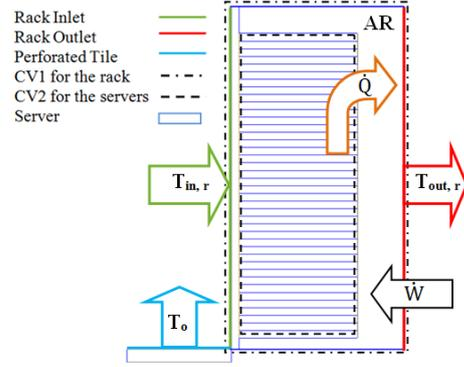
Figure 2. The schematic of the rack unit
