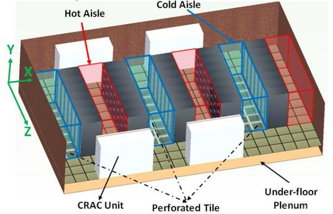
Figure 4. Orthographic view of the data centre
