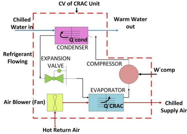
Figure 3. Thermodynamic cycle of the CRAC unit
